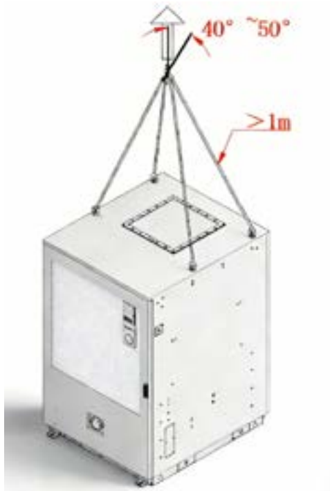
Figure 5- 7 Lifting Installation requirement
