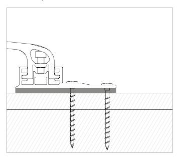
If the roof hook is underlaid for height compensation, the underlay must only be so high that the thread of the screw is still completely seated in the rafter timber and not, for example, in the underlay timber, as this cannot introduce tensile and transverse forces into the roof structure.
