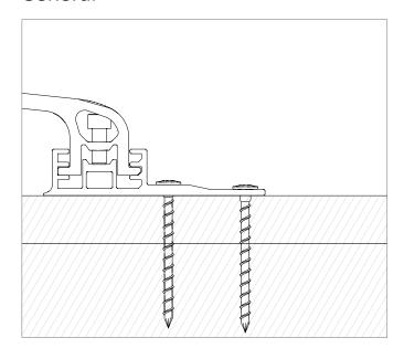
At least 2 screws must always be used to fasten a roof hook to the wooden substructure. The screws may be screwed with pre-drilling or without pre-drilling.
