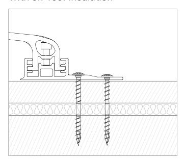
If on-roof insulation is present, the screw length must be selected so that the minimum screw-in depth of the screw in the rafter wood is maintained.
